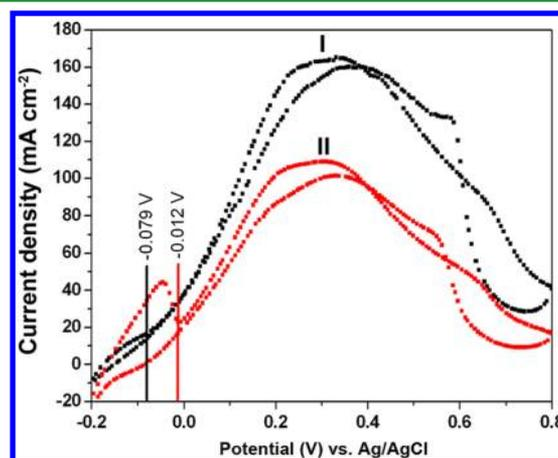
**Figure 4.** Cyclic voltammograms of the (I) PdCu/MWCNTs catalyst, (II) Pd/MWCNTs catalyst in 0.5 M  $\text{H}_2\text{SO}_4$  + 0.5 M  $\text{CH}_3\text{OH}$  aqueous solution.
