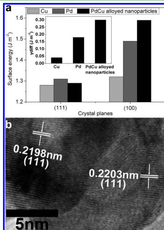
**Figure 2.** (a) Surface energies of the (111) and (100) planes of the Cu, Pd, and PdCu alloyed nanoparticles. Inset: the  $\gamma_{\text{diff}}$  between (100) and (111) planes of the Cu, Pd, and PdCu alloyed nanoparticles. (b) HRTEM image of the PdCu/MWCNTs.
