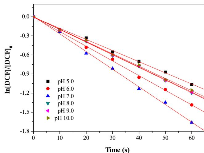
Fig. 2. Plot of  $\ln([\text{DCF}]/[\text{DCF}]_0)$  vs. reaction time under different pH conditions.  $[\text{DCF}]_0 = 3.00 \mu\text{M}$ ,  $[\text{ClO}_2]_0 = 18.9 \mu\text{M}$ ,  $\text{pH} = 7.0$ ,  $T = 298 \text{ K}$ .
