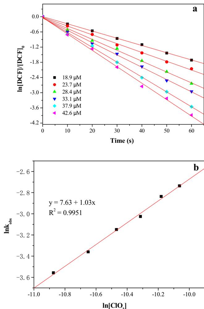
Fig. 1. Determination of reaction order for DCF oxidation by  $\text{ClO}_2$ : (a) plot of  $\ln([\text{DCF}]/[\text{DCF}]_0)$  vs. reaction time at different initial  $\text{ClO}_2$  concentrations; and (b) plot of  $\ln(k_{\text{obs}})$  vs.  $\ln[\text{ClO}_2]_0$ .  $[\text{DCF}]_0 = 3.00 \mu\text{M}$ ,  $\text{pH} = 7.0$ ,  $T = 298 \text{ K}$ .
