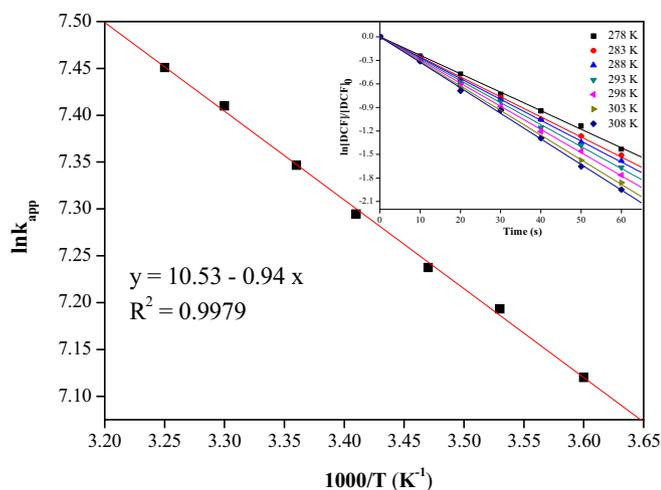
**Fig. 3.** Arrhenius plot of  $\ln k_{app}$  vs.  $1/T$  (insert: plot of  $\ln[DCF]/[DCF]_0$  vs. reaction time under different temperature). [DCF]<sub>0</sub> = 3.00 μM, [ClO<sub>2</sub>]<sub>0</sub> = 18.9 μM, pH = 7.0.
