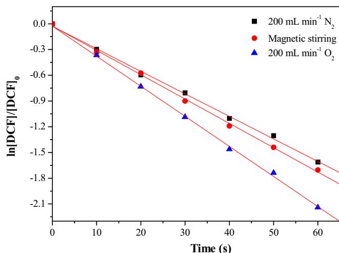
Fig. 4. Kinetics of DCF oxidation by  $\text{ClO}_2$  at various dissolved oxygen contents.  $[\text{DCF}]_0 = 3.00 \mu\text{M}$ ,  $[\text{ClO}_2]_0 = 18.9 \mu\text{M}$ ,  $\text{pH} = 7.0$ ,  $298 \text{ K}$ .
