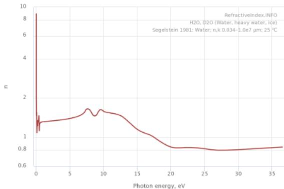
Refraction index  $n$  as a function of frequency(Hz)/photon energy(eV).
